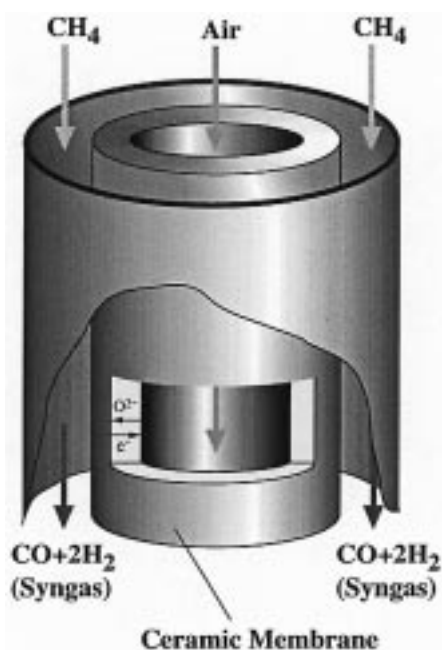
Fig. 1. Schematic drawing of oxygen-permeable membrane used in methane conversion reactor.
